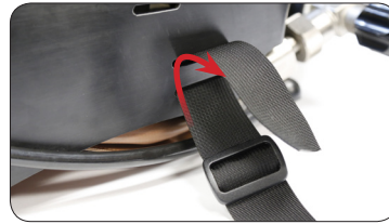
13.) Weave Adjustment Straps through the existing carrying slots in the Rebreather in all four locations.
