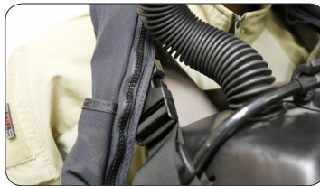
16.) Once the PlateFrame is on, attach the Adjustment Straps to the top left and right of the Rebreather system.
